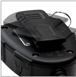
Clothing clip. 360° Rotation with positive dent stop every 45°
